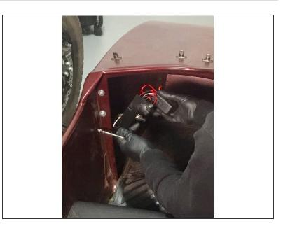
If equipped, remove the two screws securing the 12V accessory fuse panel. Place the fuse panel to the side momentarily.
