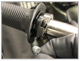
Separate the two halves of the throttle/switch housing and remove the throttle cable from the throttle sleeve.
