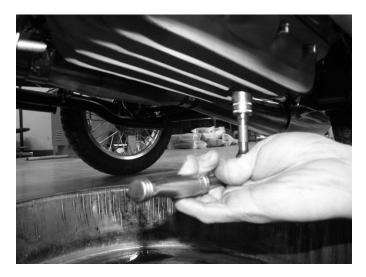
**Step 1**Place a drain pan under the oil sump and remove the drain plug using a 17mm socket
