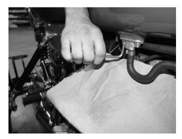
**Step 6**Remove the in-tank screen filter.
