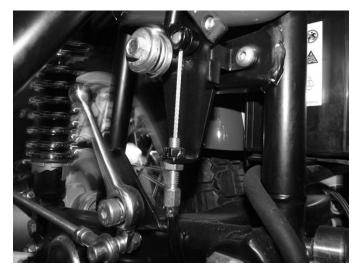
**Step 1**Locate the cable adjuster connected to the parking brake handle and be sure the parking brake is in the "off" position.
