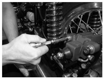
**Step 3**Remove the caliper retaining bolts and brake pads.
