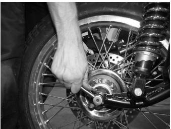
**Step 8** Tighten the axle by rotating counter-clockwise.
