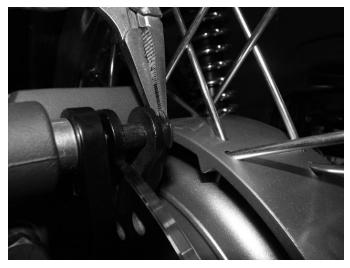
**Step 12**Re-install the caliper retaining bolt safety clips.
