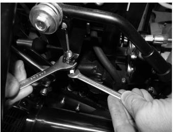
**Step 2** Adjust the cable to remove excess free play.
