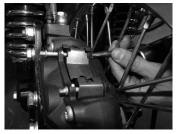
**Step 2**Carefully drive the retaining pins out of the caliper using a small punch or drift.
