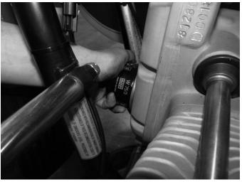
**Step 2** With the drain pan in place remove the oil filter.
