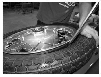
Using the provided tire spoons in your tool kit carefully remove one side of the tire from the rim.
