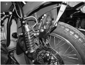
**Step 2**Carefully support the brake caliper using a strap.
