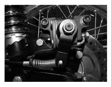
**Step 3**With the parking brake set you will have approximately 12mm between the caliper stop bracket and the brake arm with spring.
