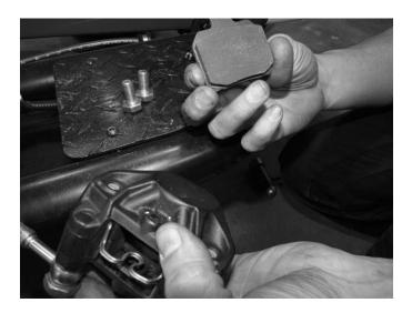
Step 4 Remove the brake pads by pulling them out of the bottom of the caliper.
