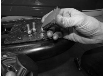
Inspect the brake pads and replace as needed.
