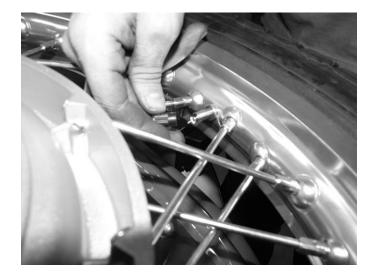
**Step 1**Remove the valve stem and deflate the tire.
