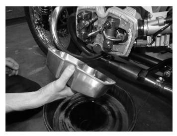
**Step 1**Starting with the left side cylinder, remove the valve cover and clean any contaminates found inside with a shop towel.
