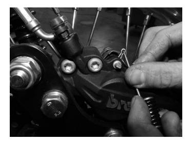
**Step 1**Remove the retaining pin safety clips.
