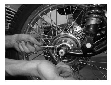
**Step 9** Tighten the axle pinch bolts to specification.
