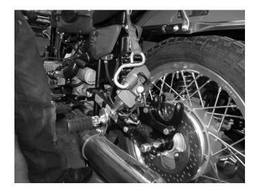
**Step 4**Support the brake caliper using a strap.
