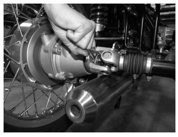
**Step 6**Remove the rear axle nut.
