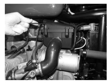
**Step 1**Remove the four retaining bolts form the air
