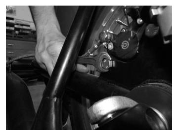
**Step 1**Remove the caliper mounting bolts.
