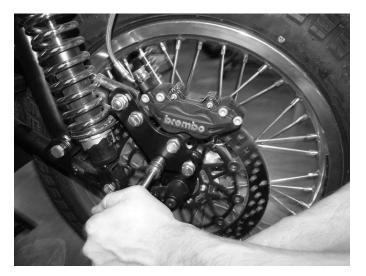
**Step 1**Remove the lower caliper mounting bracket bolts.
