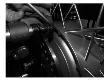
**Step 1**Remove the caliper retaining bolt safety clips.
