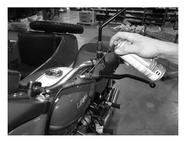
All cables including the clutch, speedometer, throttle, and parking brake cables should be lubricated with cable lube or WD-40 per the maintenance intervals. You should also lubricate all cables before and after extended periods of storage and/or after off road use.
