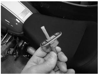
Clean all debris for the intake filter and re-install in the tank.
