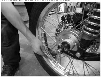
The wheel spokes should be checked on a regular basis and per the maintenance intervals.
