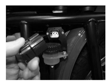
The ECU Data port is located behind the left side panel. This data port is intended for:
