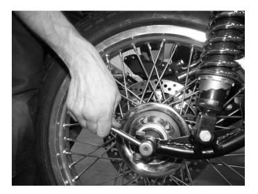
**Step 4**Loosen the axle by rotating clockwise and remove from the wheel.
