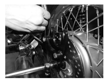
**Step 10**Torque the caliper mounting bracket bolts to specification.
