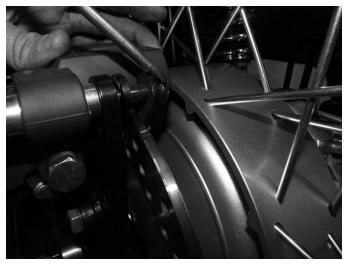
**Step 2**Carefully remove the caliper retaining bolt safety clips.
