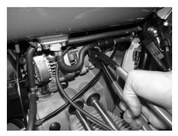
**Step 8**Install the new in-line fuel filter and replace all one-time use clamps.
