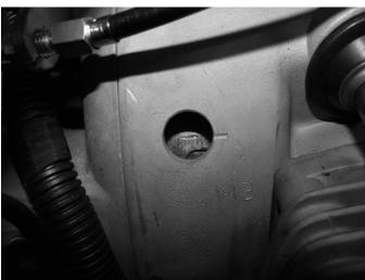
Remove the timing plug located on the right side of the engine case. Slowly rotate the engine using the kick start lever until both valves are closed and the TDC (top dead center) mark located on the flywheel is centered in the
