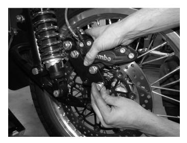
**Step 7**Re-attach the caliper with mounting brackets and tighten to specification.
