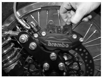
**Step 3**Remove the brake pads by pulling them out the top of the caliper.
